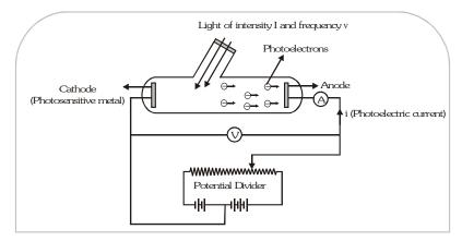
(i) Variation of photoelectric current with potential difference : With the help of the above experimental setup, a graph is obtained between current and potential difference. The potential difference is varied with the help of a potential divider. The graph obtained is shown below.
